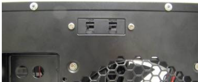
Rear fan control panel
